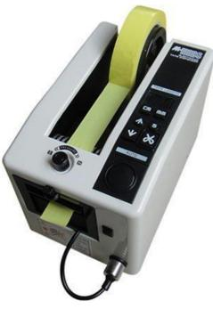
Display 3-digit digital display Applicable Tape Width 7–50mm Tape Dimension Setting Range Auto, free setting 20–999mm Motor DC motor to drive the tape and cutting knives Power 18W Power Supply AC 110V/60Hz AC 220V/50Hz Ambient Temp. 5–40 degree Ambient R. Humidity Less than 80% RH Dimensions 137W x 218D x 150H Weight 2.4kg *Fit for cutting adhesive tape, double-sided tape.*  $\Box$  Accepts tape widths from .28" to 2" (7 to 50mm)
