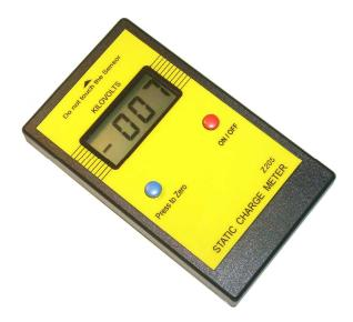
The **Static Charge Meter Z205** is a non-contact, light weight **digital** instrument designed to measure static voltages on objects & surfaces. It features a large LCD display to indicate the magnitude and polarity of the electrostatic charge directly in Kilovolts.
