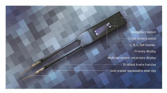
The world first handheld LCR-meter, Smart Tweezers LCR-meter is a small and light tool designed use in Surface Mount Technology (SMT). This design combining a set of tweezers tips, an LCD and an LCR-meter completely transformed the way to evaluate components. Easy one hand operation leaves the other free for other tools.
